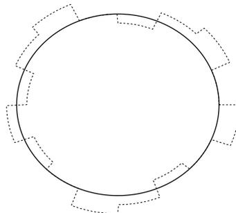
Fig 1: A discretized compensation plan (dashed-line) to the nominal boundary (solid line).
