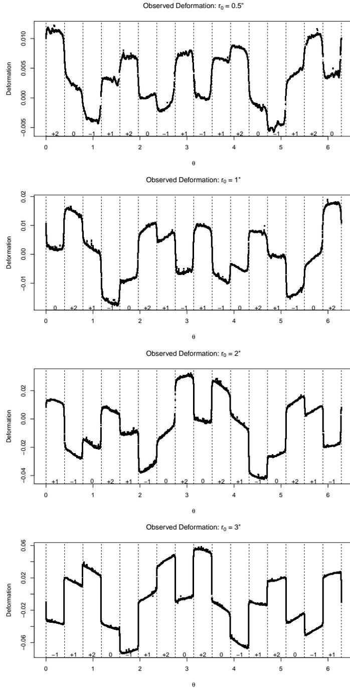
Fig 5: Observed deformations in the experiment. Dashed lines represent sections, and numbers at the bottom of each represent assigned compensations.
