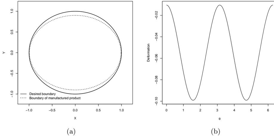
Fig 2: **(a)**: Ideal shape (solid line) vs. the actual shape (dashed-line).
