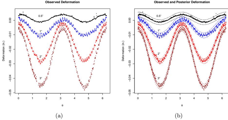
Fig 3: **(a)**: Observed deformation for  $r_0 = 0.5, 1, 2,$  and  $3$  inches, when no compensation is applied. **(b)**: Comparison of observed data with posterior predictions. Bold solid lines denote posterior means, and dashed lines the 2.5% and 97.5% posterior quantiles for each angle. These are Figures 6 and 10 in (Huang et al., 2013).
